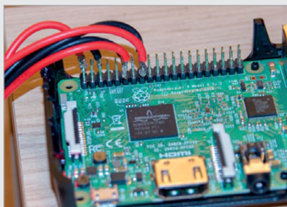
Above The power and data wires are soldered to the Raspberry Pi 3 and the software was installed to a 16GB card
