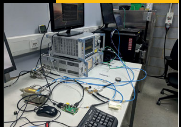
Below Conformance testing for 5 GHz WiFi was a challenge for the new radio hardware
