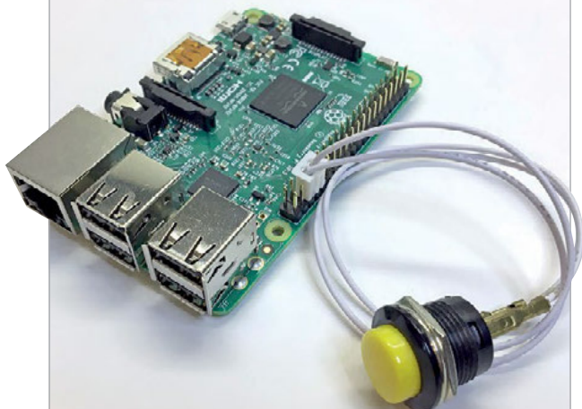
Phillip's script includes ways to disable read-only mode, by use of a jumper or quick button connect
