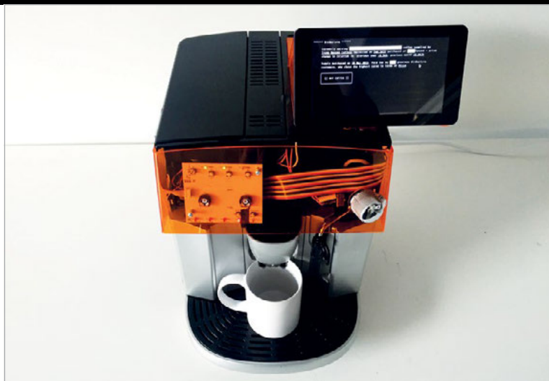
Above The technology is advanced, but BitBarista is built using a standard De'Longhi coffee maker
