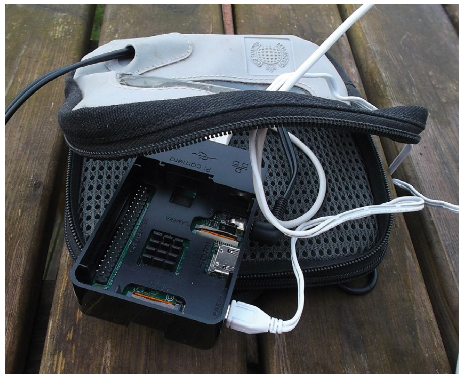
Above The Raspberry Pi handles the conversion of text in webpages to speech
