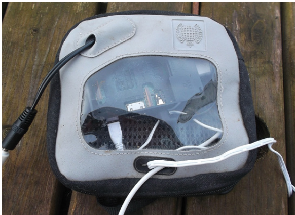
Above An outer case may be used to protect the Raspberry Pi
