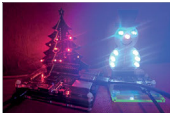
Above As a Christmas decoration, we used the Pi Hut 3D Xmas Tree and Ryantek SnowPi boards together by plugging a Pi Zero into a Pi 3
