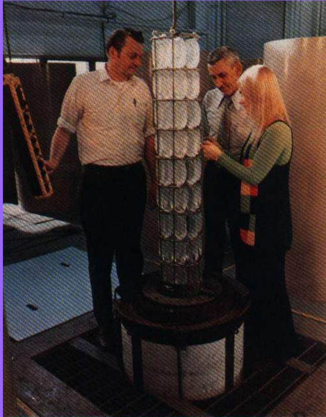
*A cluster of synthetic quartz crystals is harvested from a production autoclave at AT&T Network Systems plant*
