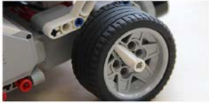
The white pointers on the EV3's tires help you to see how much the wheels are rotating.
